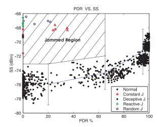
Figure 6: The (PDR,SS) measurements, indicating the relationship between PDR and signal strength. Also presented are the (PDR,SS) values measured for different jammers. The data was binned into three PDR regions, (0,40), (40,90) and (90,100), and the corresponding 99% confidence intervals are presented. The shaded region is the jammed-region, and corresponds to (PDR,SS) values that are above the 99% signal strength confidence intervals and whose PDR values are less than 65%.
