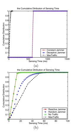
Figure 5: The cumulative distribution for the carrier sensing times measured using MICA2 Motes.
