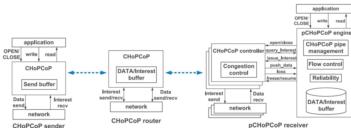
Fig. 4. pCHOCoP protocol architecture. The pCHOCoP receiver consists of a pCHOCoP engine and multiple CHOCoP controllers.
