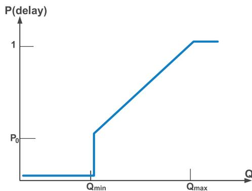
Fig. 3. Delay probability function for FISP.
