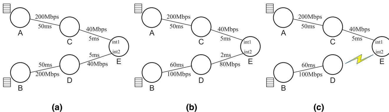
Fig. 10. Three multi-homing topologies. Each consists of two sources (A and B), and the receiver E requests content from them using both of its interfaces.
