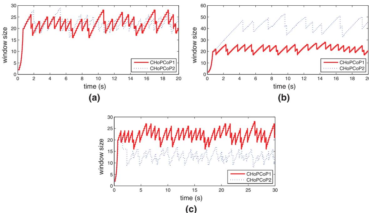
Fig. 12. The receiver window size of the two CHoPCoP pipes at the three multi-homing topologies.
