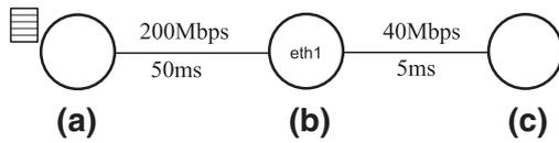
Fig. 5. A three node baseline topology, consisting of a source (A), a router (B) and a receiver (C).
