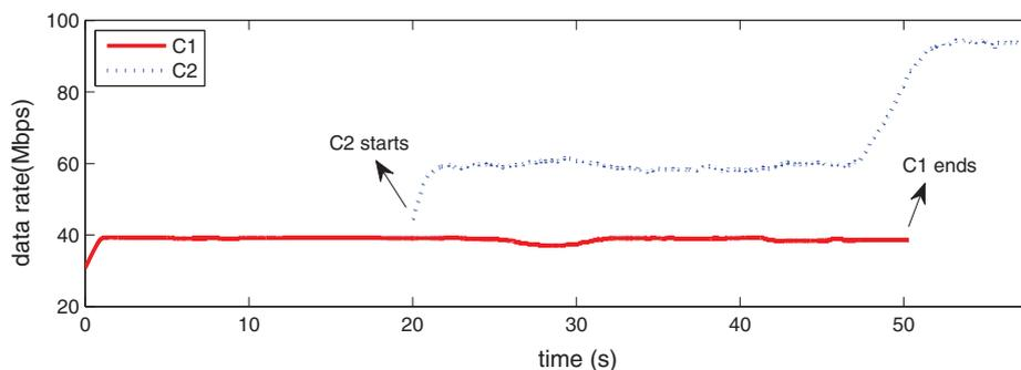
**Fig. 9.** The receiving rate for the two receivers. F initiates content flow  $C_1$  (with source A) while G initiates content flow  $C_2$  with two sources A and B.
