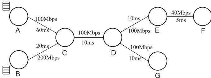
**Fig. 8.** A larger-scale topology with two sources (A and B) and two receivers (F and G). Link EF is the bottleneck link between A/B and F, while link CD is the bottleneck between A/B and G.
