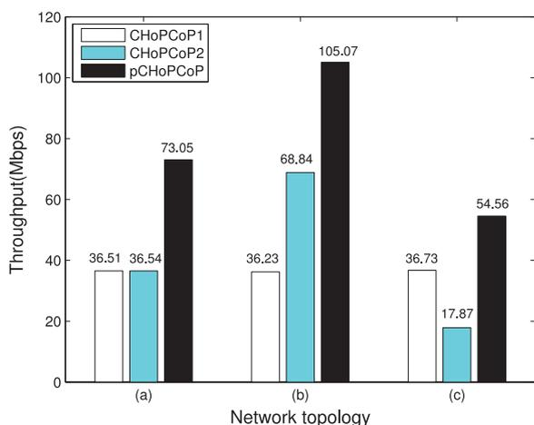
Fig. 11. The throughput of the two CHoPCoP pipes and the aggregated pCHoPCoP at the three multi-homing topologies.
