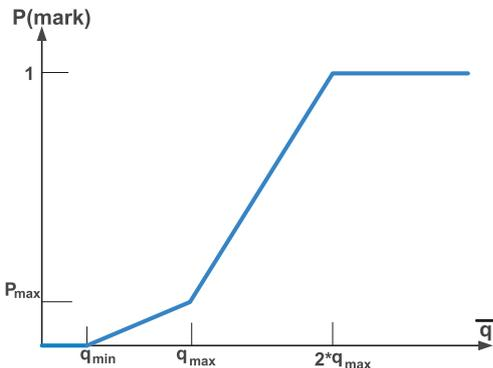
Fig. 2. Mark probability function for REM.
