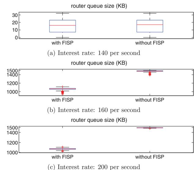
Fig. 7. Boxplot of router queue size with and without FISP under different CIR. At a low CIR, both schemes perform similarly. At a high CIR, FISP nicely controls the router queue size, and thus avoids queue overflow. Without FISP, the router queue overflows when the CIR is above 160 Interests per second.
