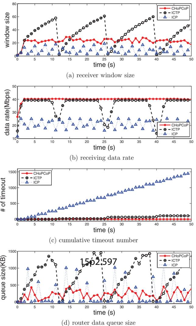
Fig. 6. The performance results for a 3-node baseline topology. ICP and HR-ICP behave very similarly, we thus use the ICP curve to represent both schemes.
