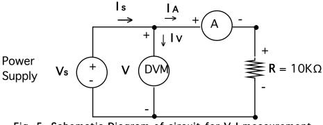
Fig. 5 Schematic Diagram of circuit for V-I measurement
