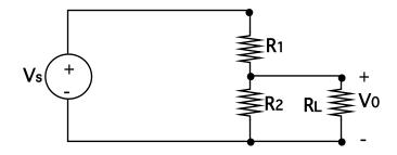
Fig. 3 A Voltage Divider Connected To A Load Of R<sub>L</sub> ohms
