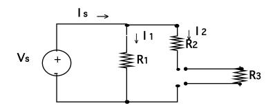
Fig. 7 A Current Divider Circuit
