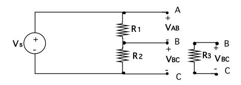
Fig. 6 A Voltage Divider Circuit
