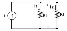
Fig. 4 A current Divider Circuit
