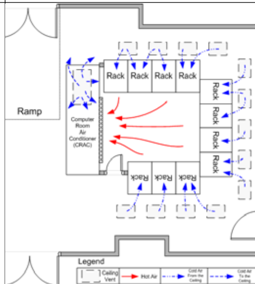
Figure: At far left, a schematic of the temperature-profiling equipment deployed at the Rutgers University datacenter. At near left, a floor plan of the machine room depicting airflow patterns.
