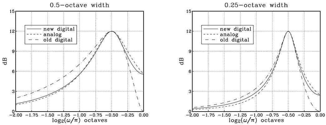
Fig. 8 Center frequency  $\omega_0 = 2^{-0.5}\pi$ . Octave widths  $\Delta\gamma = 0.5$  and  $\Delta\gamma = 0.25$ .
