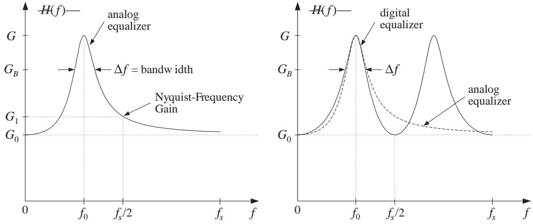
Fig. 1 Conventional analog and digital equalizers. Digital design has  $G_1 = G_0$  at  $f_s/2$ .
