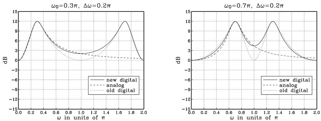
Fig. 5 12-dB boost at  $\omega_0 = 0.3\pi$  and  $\omega_0 = 0.7\pi$ . Bandwidth  $\Delta\omega = 0.2\pi$  is measured at 9 dB.
