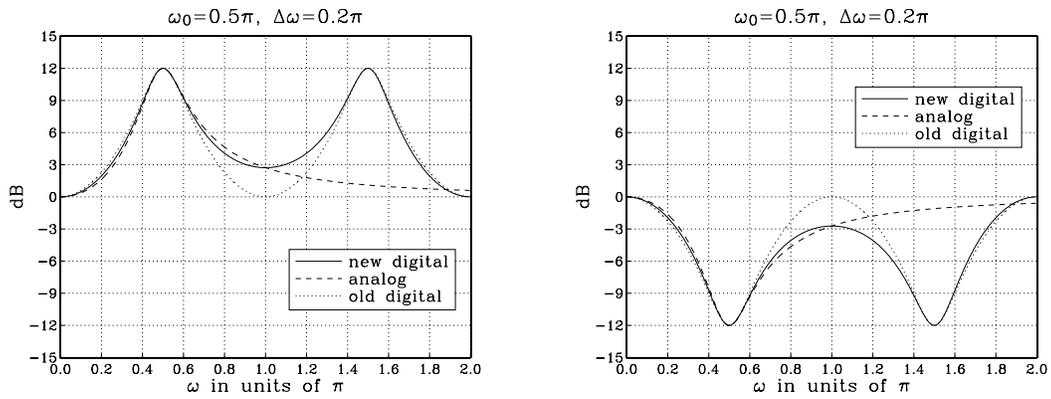
Fig. 4 12-dB boost and cut at  $\omega_0 = 0.5\pi$ . Bandwidth  $\Delta\omega = 0.2\pi$  is measured at  $\pm 9$  dB.
