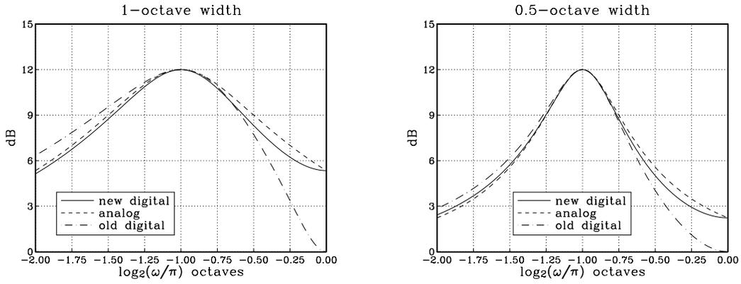
Fig. 7 Center frequency  $\omega_0 = 2^{-1}\pi$ . Octave widths  $\Delta\gamma = 1$  and  $\Delta\gamma = 0.5$ .
