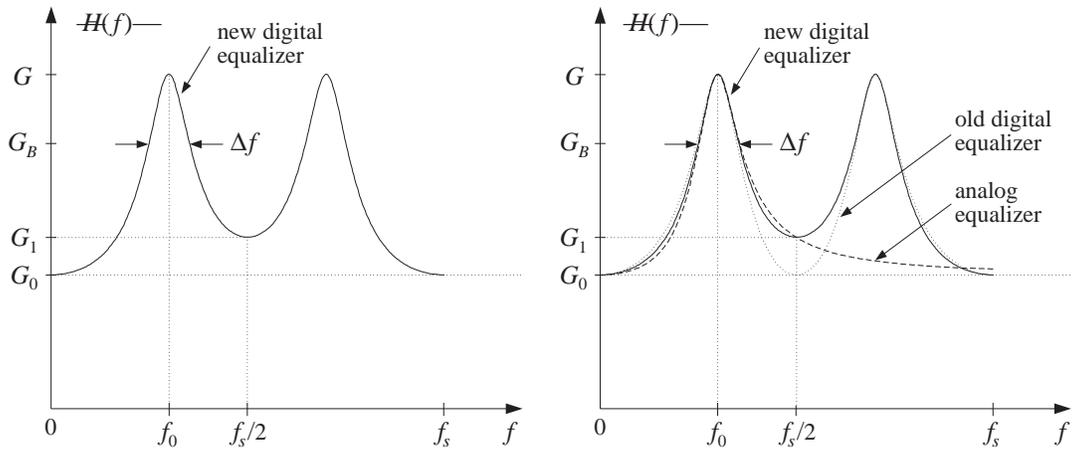
Fig. 2 New digital equalizer matches the Nyquist-frequency gain of the corresponding analog equalizer.
