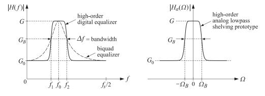
**Fig. 1** Specifications of high-order equalizer and the equivalent lowpass analog prototype.
