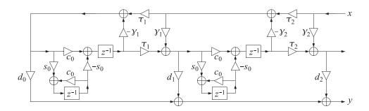
Fig. 6 Frequency-shifted normalized lattice realization of the sections of Eq. (18b).
