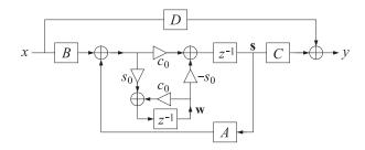
Fig. 7 Frequency-shifted state-space realization of the filter sections of Eq. (18b).
