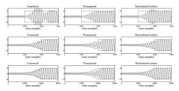
Fig. 16 Sinusoidal response of equalizer with time-varying gain.
