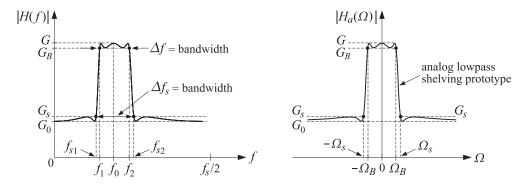
Fig. 3 Design specifications of elliptic equalizer and corresponding shelving filter.
