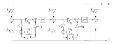
Fig. 5 Frequency-shifted transposed realization of the filter sections of Eq. (18b).
