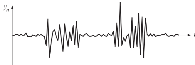
Fig. 1.11.1 Piece-wise stationary signal.
