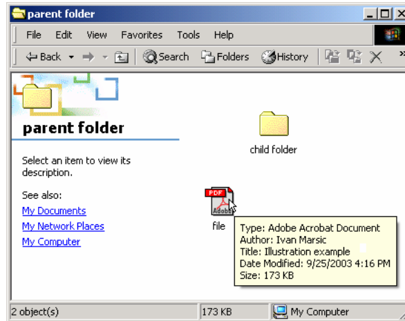
Fig. 5. Example of a gesturing in the user interface. By rolling the mouse cursor over a file's icon (pointing gesture), the user can reveal essential metadata about the file. Notice that there is no manipulation involved.
