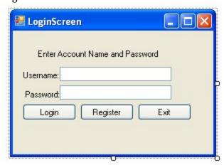
The login screen allows a user to login using an existing account, create a new one, or exit the program. Login and Register require two text entries and a button click, the exit button only requires one click. AccountScreen:
