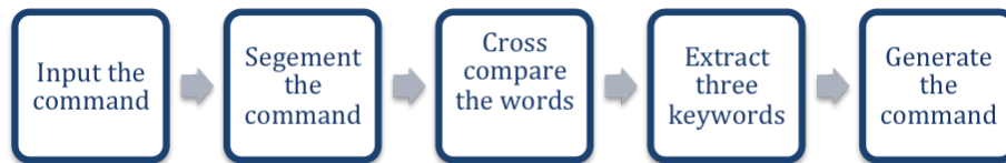
Figure 83: The algorithm of keywords extraction
