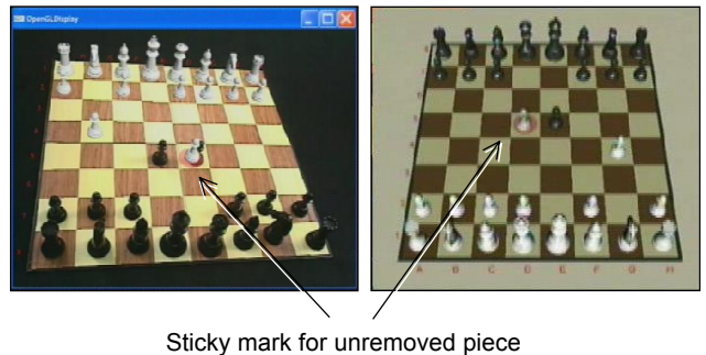
Figure 5. Visual cue for notifying the novice to remove a piece. The black piece (real in novice view), captured by the white pawn, has a sticky red spot below
