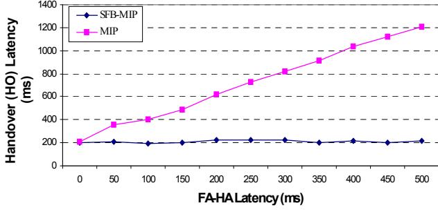
Fig. 7. Latency comparison with MIH support
