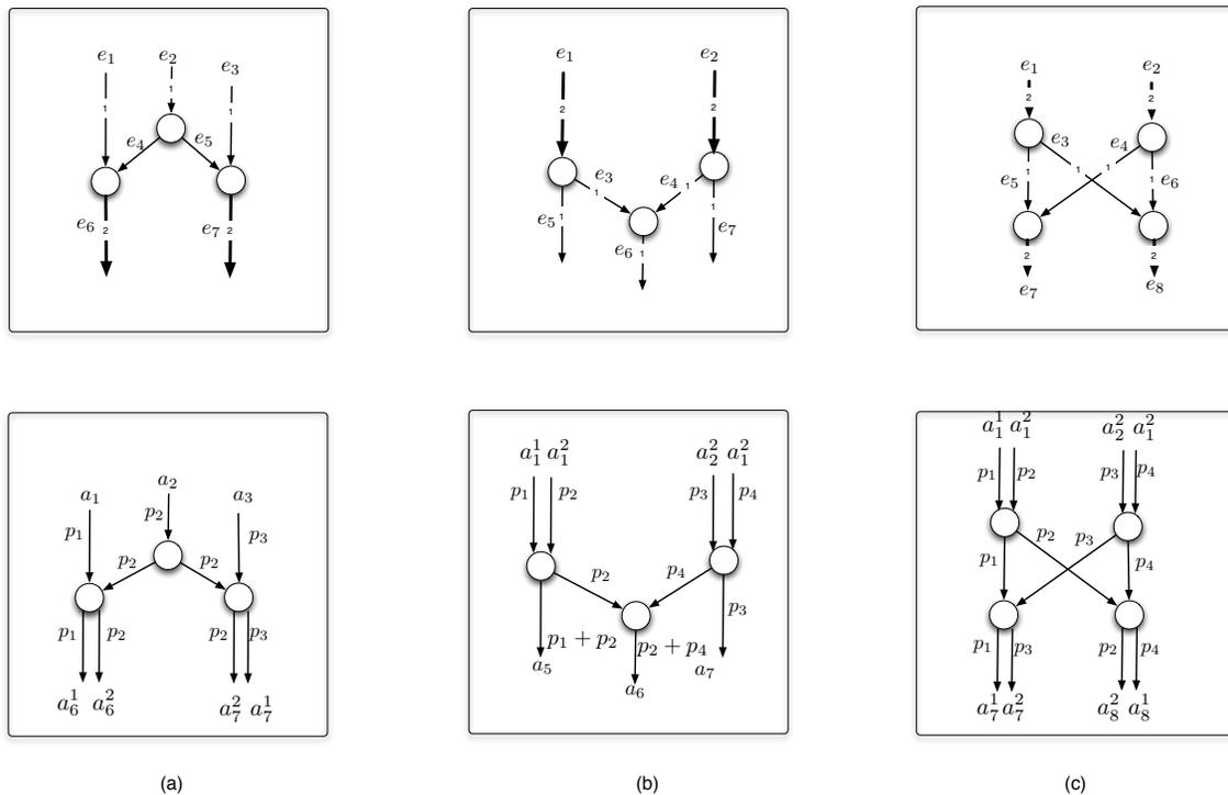
Fig. 9. Network code for simple unicast networks: (a) Encoding for blocks of Type A; (b) Encoding for blocks of Type B; Encoding for blocks of Type C.
