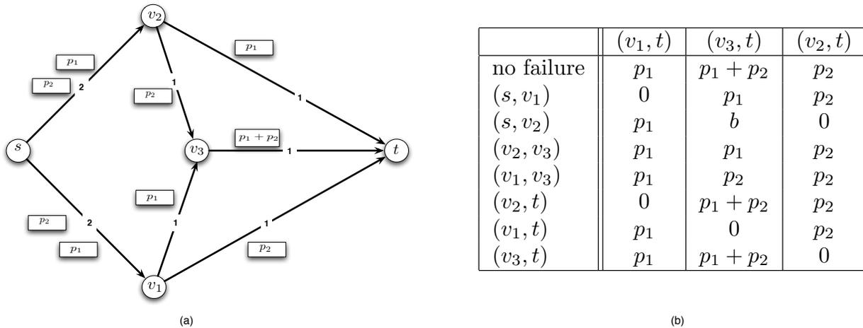
Fig. 2. (a) A network coding approach for  $h = 2$  (b) A list of the packets received by the destination  $t$  for each single edge failure scenario.
