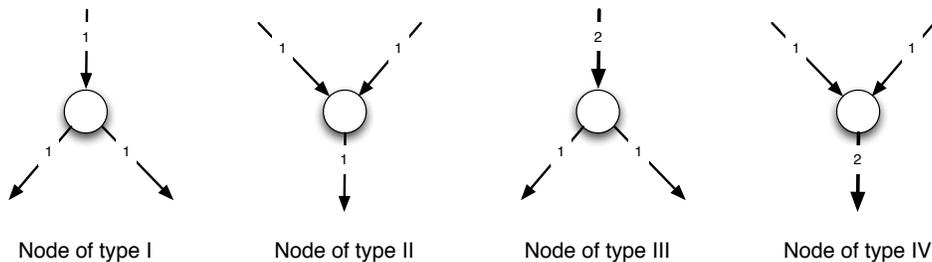
Fig. 5. The four types of nodes in a simple unicast network.
