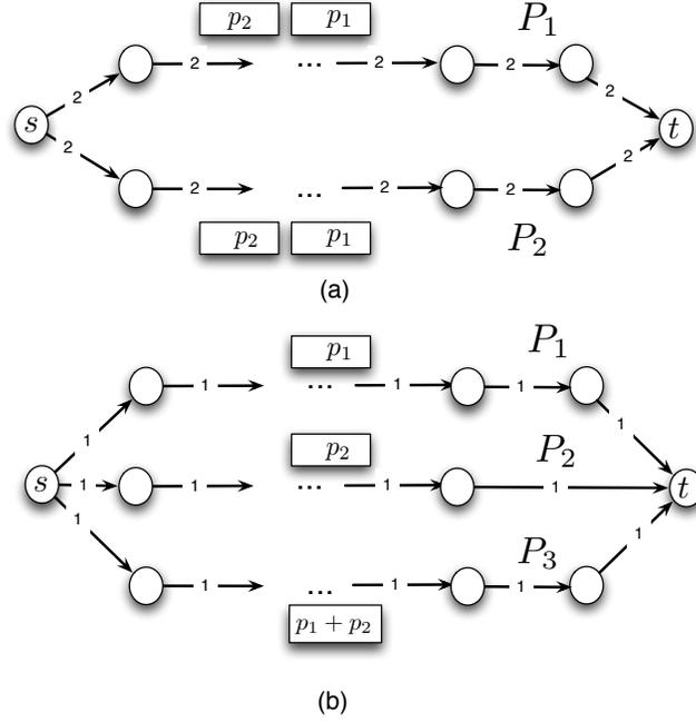
Fig. 1. (a) Dedicated path protection method (1 + 1 path protection); (b) Diversity coding method for  $h = 2$ .
